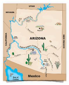
In 2001, Tucson Water began blending its groundwater with **Colorado River water** that is pumped 336 miles (541 km) from Lake Havasu via the Central Arizona Project (CAP). There are fourteen pumping stations along the CAP to help move the water from lower to higher elevations, with a gain of nearly 3,000 feet (914 m). The CAP is the largest single user of electricity in Arizona.
